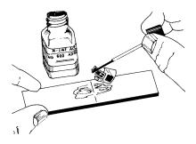
Now, by lifting at a shallow angle, peel back one end of the taped assembly so as to raise both gage and terminal. By curling this mylar tape back upon itself, it will remain in position, ready to be accurately repositioned after application of adhesive.
